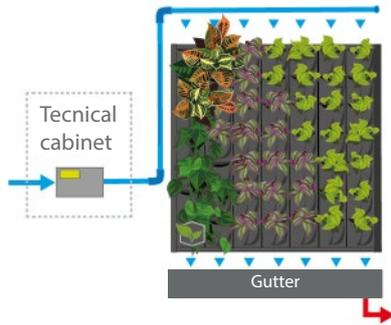
This scheme suits small and medium surfaces of vertical gardens (up to 85-90 m<sup>2</sup>). In this scheme, extra water is not left, because the system is connected right to the drain. Water and electrical supply in the technical cabinet are necessary for auxiliary installations
