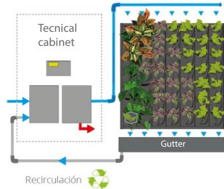
This scheme suits large and very large surfaces of vertical gardens (>90 m<sup>2</sup>). In this scheme, extra water is left for watering in a closed system connected to reservoirs, where water is reused for green wall watering after treatment. Base branches of the water line in the technical room are necessary for additional installations, reservoirs, and control.
